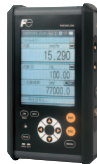
Flow transmitter (FSC)
