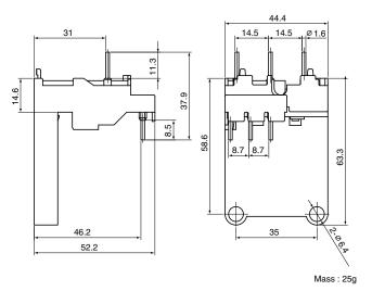
Power Connection Kit for Reversing (Insert)[Insert for Power Supply Side] [Insert for Load Side]
