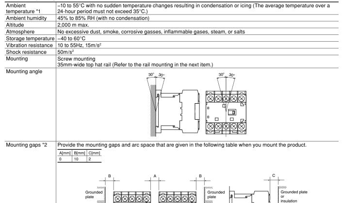
Note \*1: The ambient temperature is the temperature near the product during operation.
