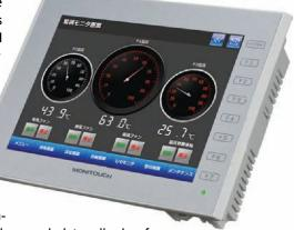
card slots, allowing for better connectivity to peripheral devices. Select models will have onboard sound output; wireless LAN (access point incorporated); and be Class 1, Division 2 rated. The VNC server function ensures that all models can be accessed from a tablet or PC, and the com-
