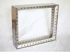
precision-formed air passages (hole pattern) that are integrated into a stainless steel assembly. Built to order, the structure's engineered hole pattern can maintain its measuring accuracy, even with 50 percent hole blockage. The system fits into existing ductwork — no duct removal is required.
