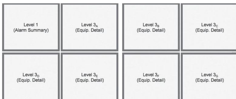
Figure 2: Typical console screen use with a like-for-like HMI migration project.
