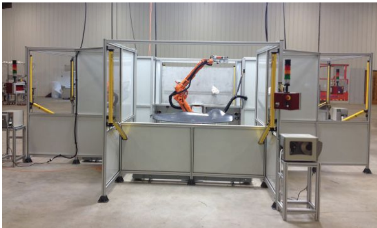
Figure 2: Fitz-Thors engineers designed this machine-vision enabled station in a workcell with a turntable used to treat smaller parts for a Tier 1 automotive application.
