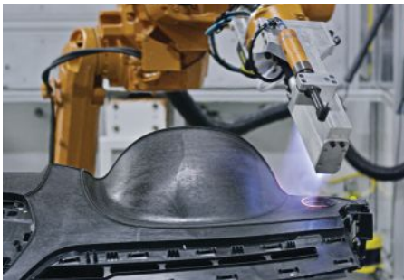
Figure 5: Configuration for this vision-enabled ABB robot is achieved via Cognex EasyBuilder user interface, by selecting the pattern find vision tool with an angle orientation limit that provides a percentage match to ensure that the right part is positioned correctly in the fixture. The ABB IRB 2600ID robot uses an Enercon Dyne-A-Flame surface treater to flame treat the parts for a Tier 1 automotive supplier.
