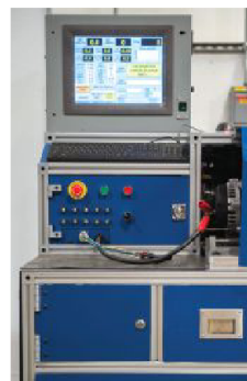
Figure 3: The test system includes a touchscreen PC running HMI software, which allows operators to select recipes and perform other interactions with the system. Opera-
