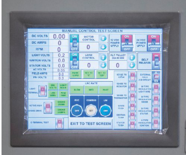
Figure 4: The touchscreen HMI is programmed to lead the operator through the test procedure by following a series of logical steps. After using the AutomationDirect Productivity3000 PAC and the Indusoft Web Studio software, other parts of MPA manufacturing and test processes are being examined for opportunities to increase production or improve quality through a higher level of automation.
