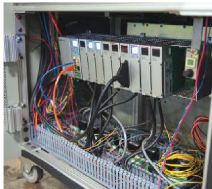
Figure 2: A programmable automation controller automates the test system, monitors its operation and gathers test data. High processing speeds, sophisticated data handling, and high-level programming options were a must to meet system requirements. A sophisticated controller is the heart of the test system, in this case an AutomationDirect Pro-ductivity3000 Programmable Automation Controller (PAC).
