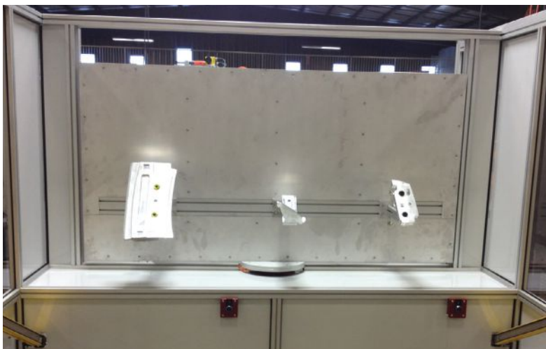
Figure 3: One of three stations in the Fitz-Thors designed robotic workcell doesn't have a turntable and is made to heat-treat larger parts. ABB SafeMove robot safety option enables operators to safely load parts on the three stations without turntables.
