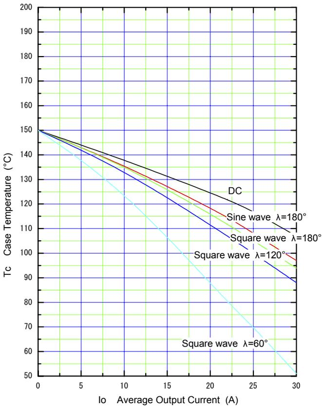
λ: Conduction angle of forward current for each rectifier element
