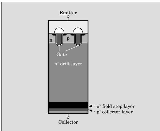
the FS-IGBT, and enables the practical utilization of a system that employs this high current density device.
