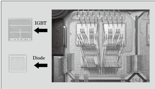
This technique is also an effective means for shrinking the chip size<sup>(2)</sup>. Figure 4 shows a conventional module structure, and the internal structure of a double-sided cooling module made by Denso and for which IGBT and diode chip double-sided cooling is possible.
