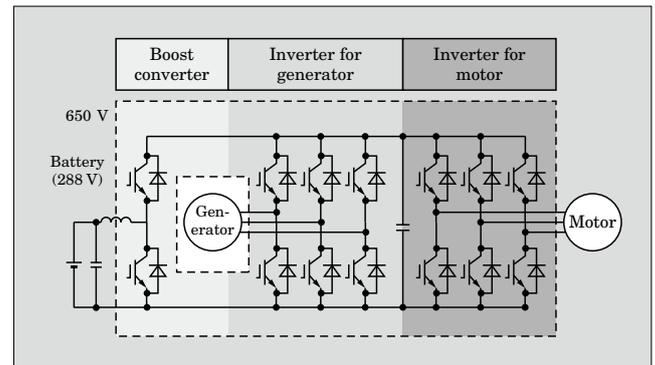
However, with this type of conventional module structure in which many power chips are arranged in a planar state, the PCU will have a large footprint, and the requirement for smaller size cannot be satisfied. Thus, it is important to reduce the number of power chips, and challenges for achieving this goal include developing a power chip capable of withstanding a high current density and achieving a significant improvement in heat dissipation performance.
