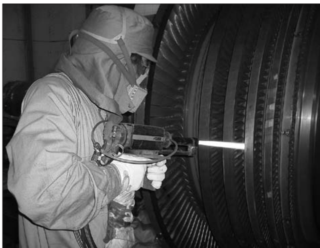
Fig.2 Spray coating of rotor
