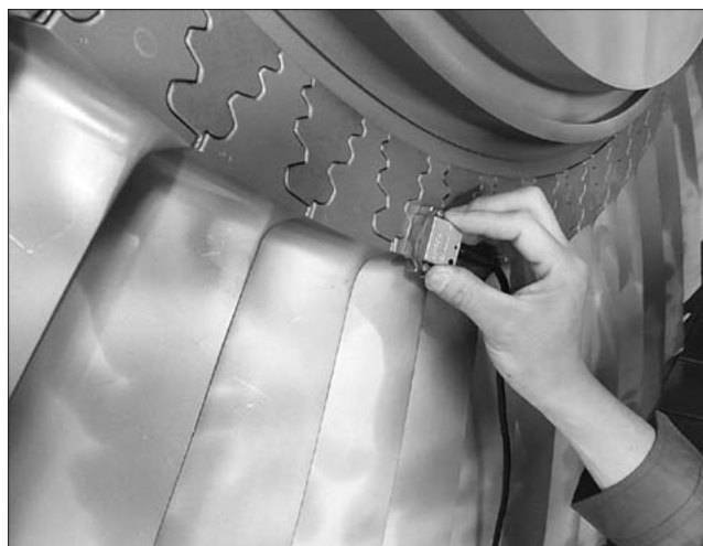
Fig.12 Phased array inspection of fir tree type root of low-pressure moveable blade
