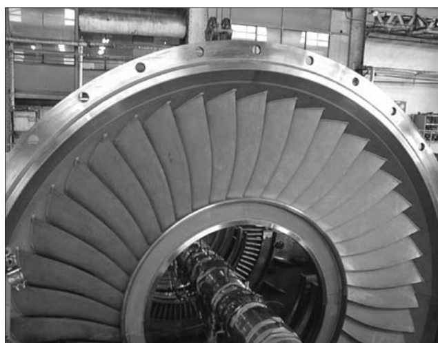
Fig.4 Lean-radial stationary blades
