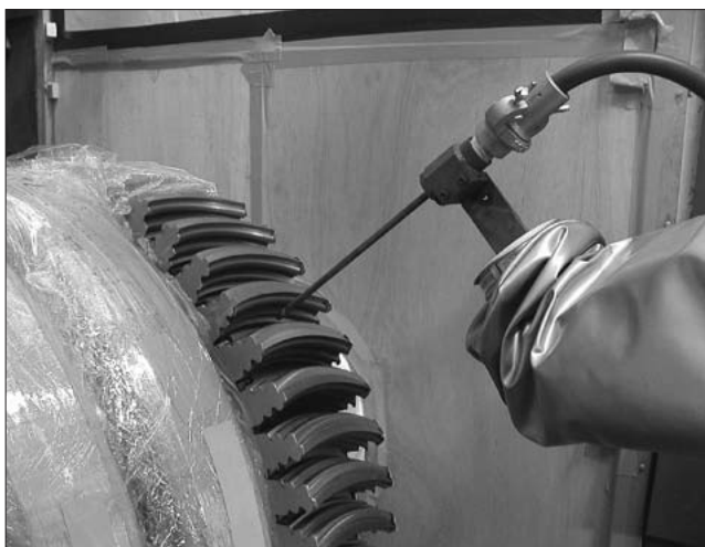
Fig.3 Shot peening of rotor blade
