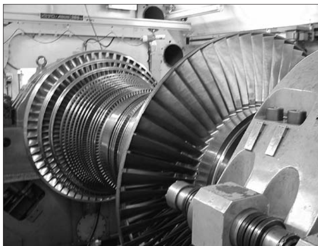
Fig.5 Rotational vibration test of new-generation low-pressure blade for geothermal steam turbine
