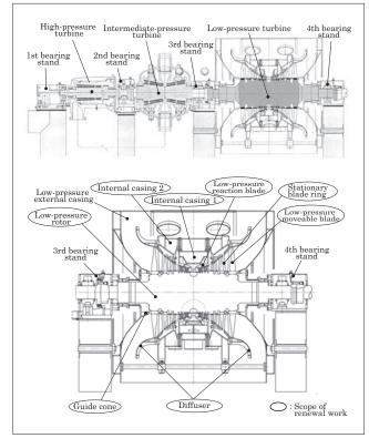
Fig.3 Reaction blades designed entirely with 3-dimensional CAD technology
