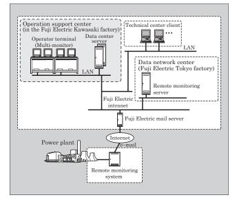
Fig.13 System configuration
