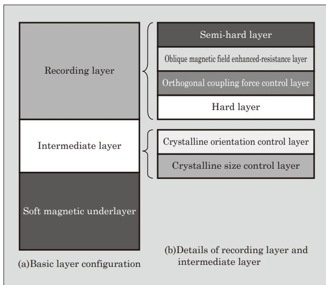
Fig.2 Basic layer configuration and details of media
