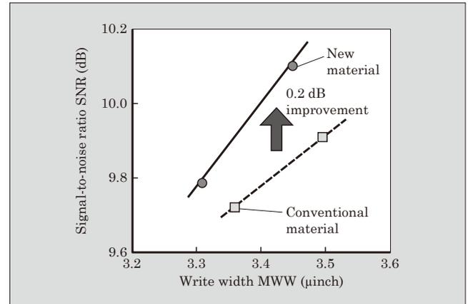
Fig.6 Change in SNR according to soft magnetic underlayer material
