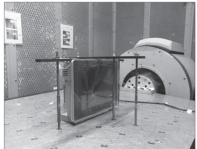
Fig.5 Acceleration resistance test circumstance
