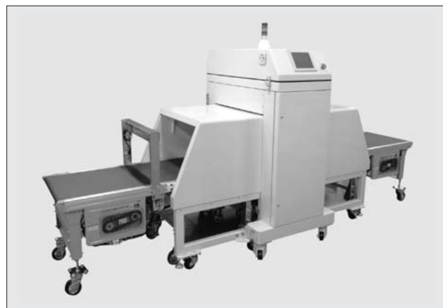
Fig.18 Radioactive contamination inspection system for monitoring foodstuff
