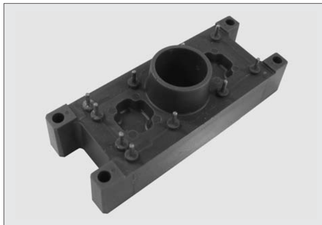
Fig.13 SiC power module package
