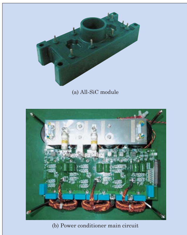
Fig.4 Application to photovoltaic power conditioner
