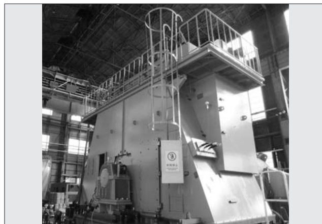
Fig.40 7,700 kW, 34P synchronous motor under factory test
