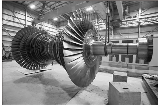
Fig.10 Geothermal turbine rotor installed
