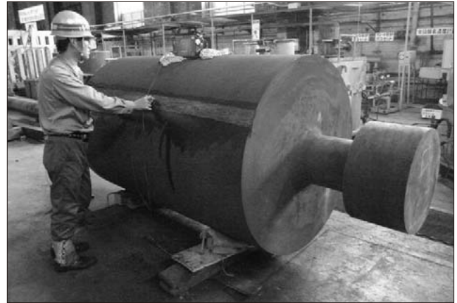
Fig.10 Improved 12% Cr steel prototype rotor
