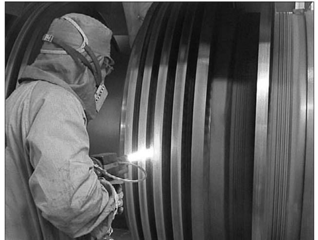
Fig.3 Coating with high velocity oxy-fuel spraying
