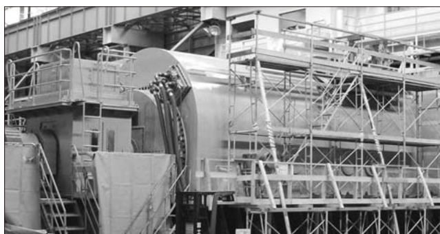
Fig.11 Global VPI insulated indirectly hydrogen-cooled turbine generator during factory testing
