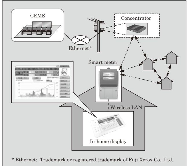
Fig.5 System configuration of smart meter
