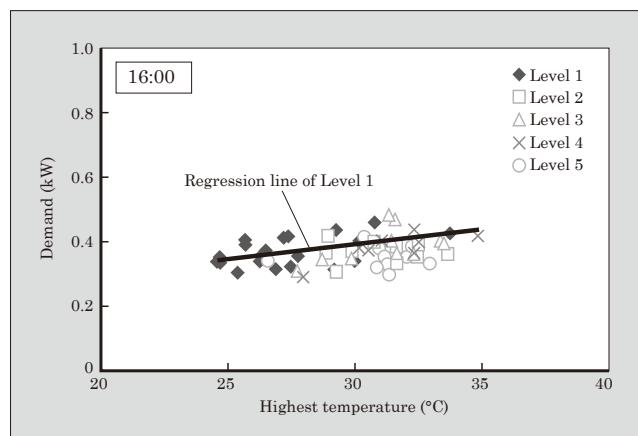
Fig.10 Relationship between the highest temperature of the day and demand at 16:00
