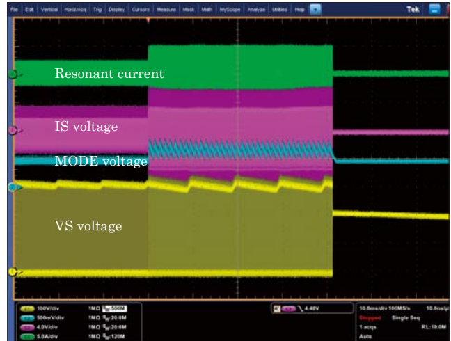
Fig.9 Waveform during over-current protection operation
