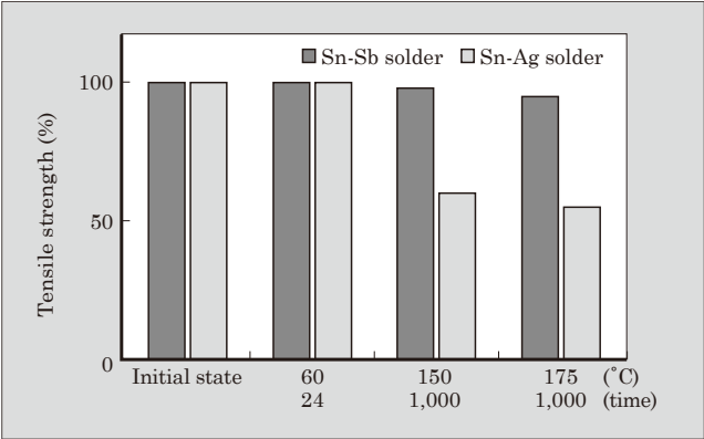
Fig.7 Tensile strength variance in solder after thermal storage test
