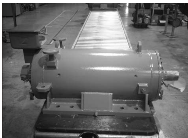
Fig.5 Large-capacity low-inertia servomotor
