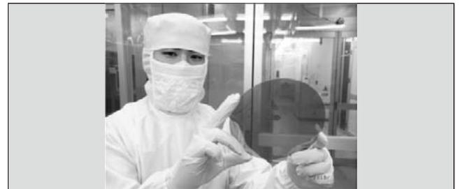
Fig.11 6-inch SiC wafer
