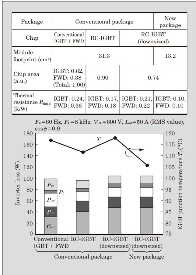
Fig.12 RC-IGBT inverter loss and IGBT junction temperature calculation results
