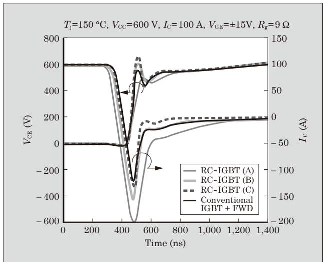
Fig.6 Reverse recovery waveforms of RC-IGBT
