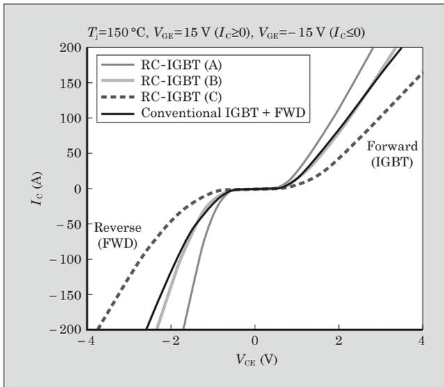
Fig.3 Output characteristics of RC-IGBT
