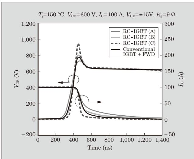
Fig.4 Turn-off waveforms of RC-IGBT
