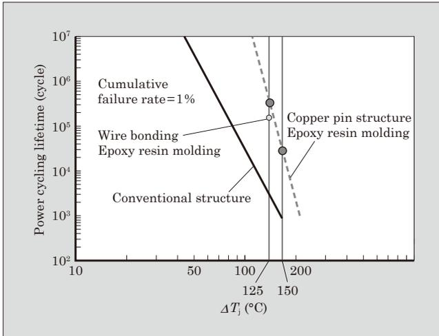
Fig.11 Power cycling lifetime of new package
