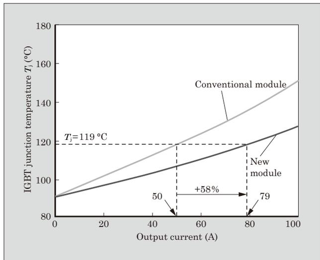
Fig.13  $T_j$  of new module
