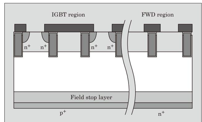
Fig.2 Cross-sectional view of RC-IGBT
