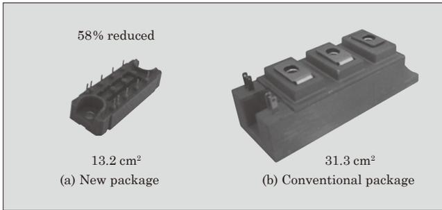
Fig.10 Footprint of new package (1,200 V/100 A)
