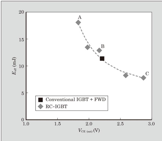
Fig.7 IGBT loss trade-off of RC-IGBT
