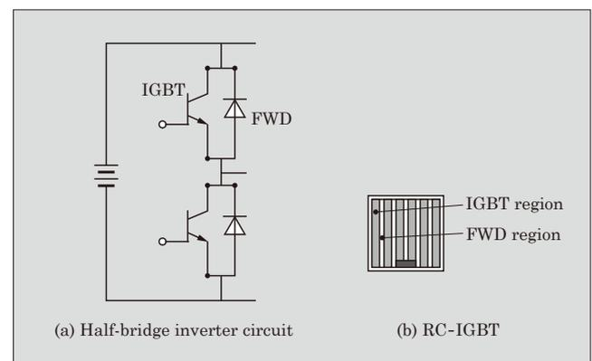
Fig.1 Half-bridge inverter circuit and RC-IGBT
