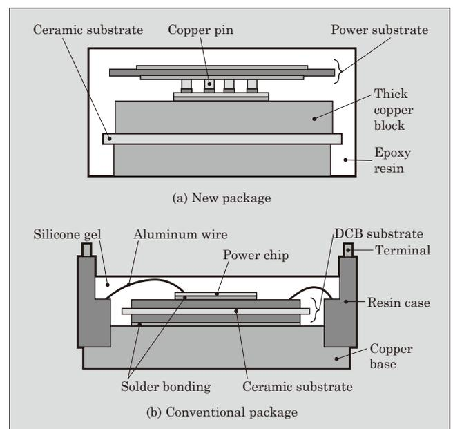
Fig.9 Cross-sectional view of new package
