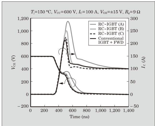
Fig.5 Turn-on waveforms of RC-IGBT
