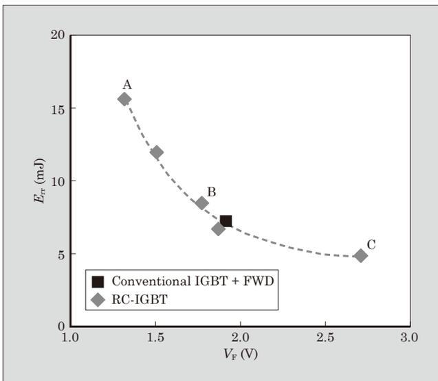
Fig.8 FWD loss trade-off of RC-IGBT
