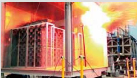
(b) Internal arc test for the switchgear (third-party certification testing)
