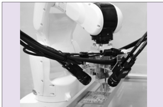
Fig. 11 Electronic component mounting using visual feedback control
