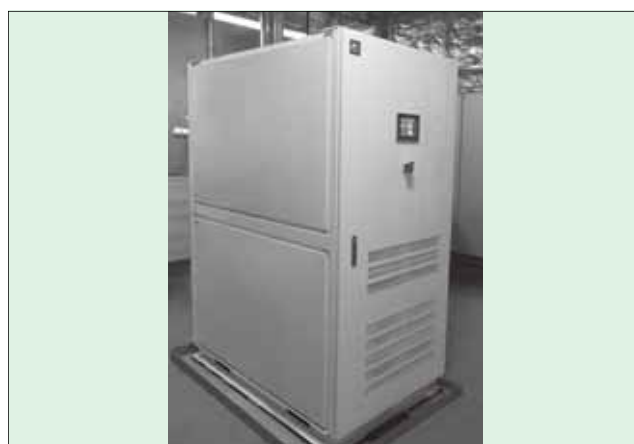
Fig. 10 Steam generation heat pump (field test machine)
