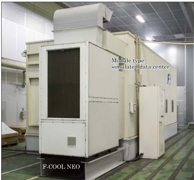
Fig.8 Hybrid air-conditioner “F-COOL NEO” evaluation equipment
