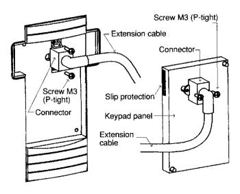
Fig. 8-2-2 Extension cable connection
