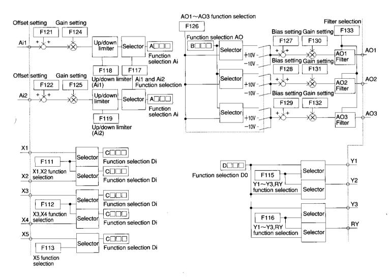
Fig. 9-2-8 Block diagram of function selection input/output selection
