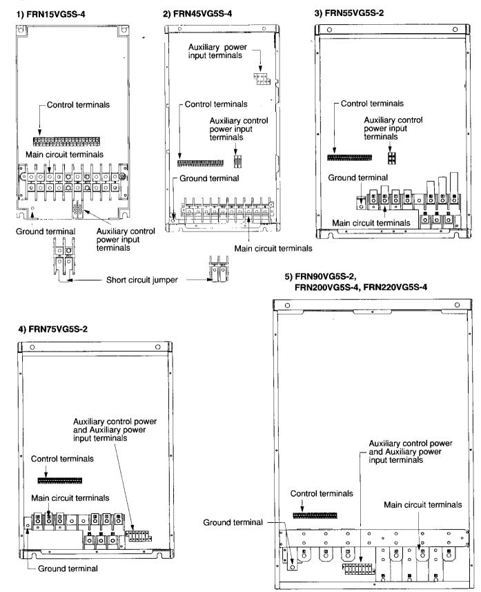
Fig. 6-1-4 Terminal arrangement
