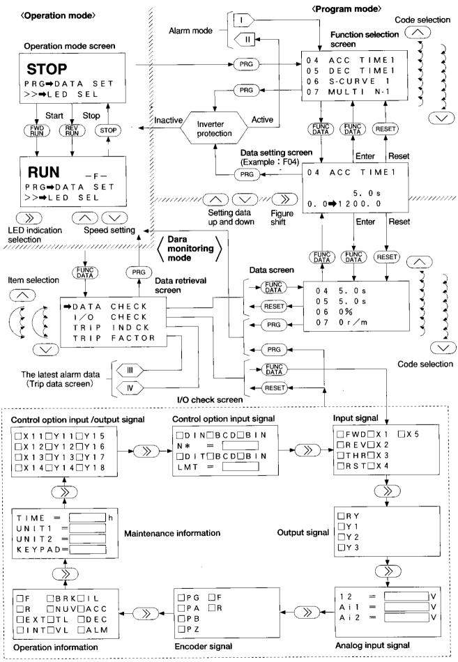
Fig. 8-3-4 keypad panel operation and LCD indication 1
