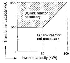
Fig.6-2-5 Application DC link reactor(1)
