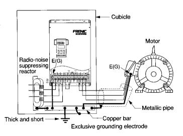
Fig. 6-3-2 Grounding of inverter system
