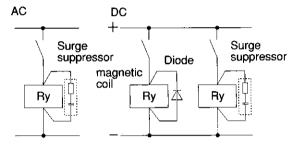
Fig. 6-5-12 Surge suppressor connections
