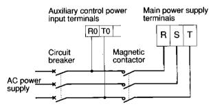
Fig. 6-2-2 Magnetic contactor connections
