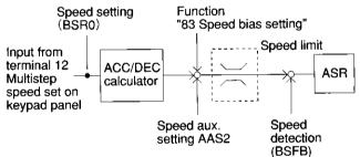
It is judged by comparing the input of ACC/DEC calculator (BSR0) with the speed detection value (BSFB) that the inverter is either in acceleration or in deceleration. The signals of in acceleration or in deceleration are made OFF at speed arrival based on the level of function "70 Speed arrival (Detection width)".
