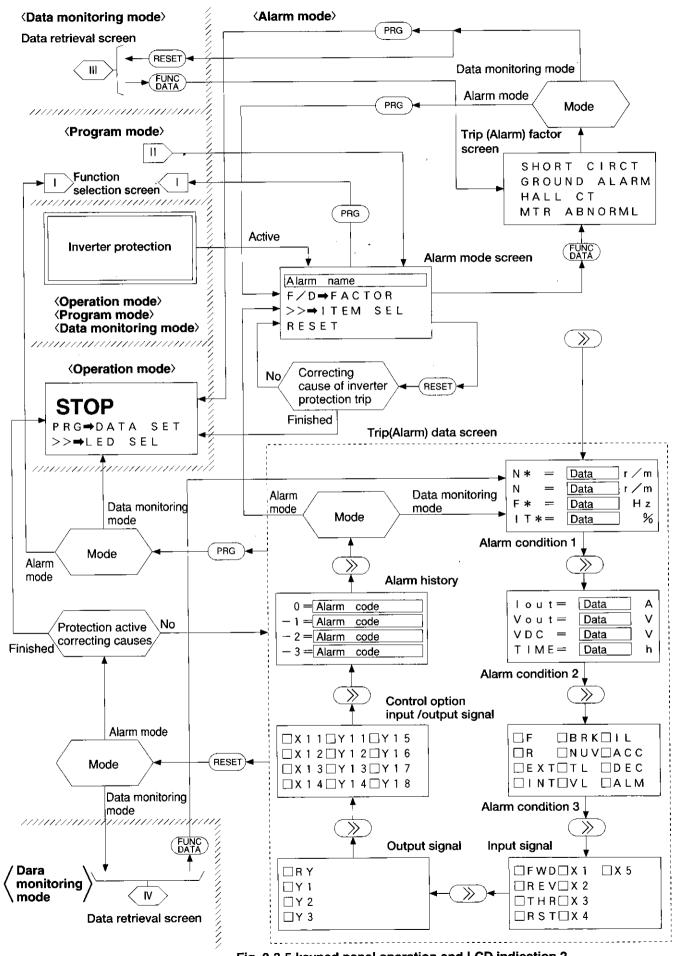
Fig. 8-3-5 keypad panel operation and LCD indication 2
