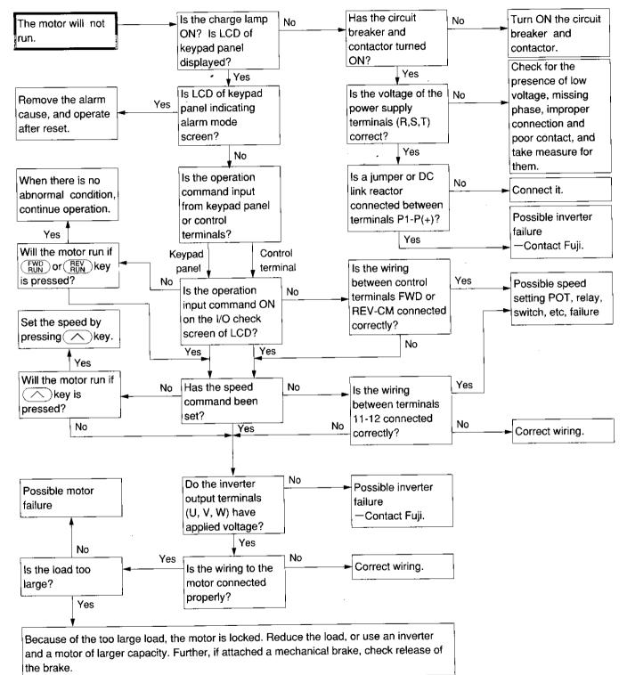
NOTE: Monitor the operation command or speed setting value on LED and LCD of keypad panel by selecting each function.
