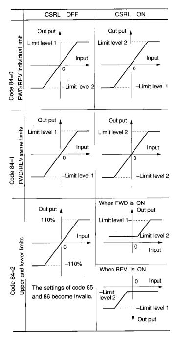
FWD/DEV individual limit can be used as a function of reversing prevention when the data are as follows:
