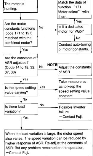
**NOTE:** In general, the hunting is made small by reducing the data of function "14 and 37 ASR (*P* constant)" and increasing the data of function "15 and 38 ASR (I constant)"
