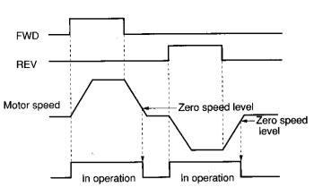
The zero speed can be also detected by the speed setting value according to function "69 Speed detection mode".
