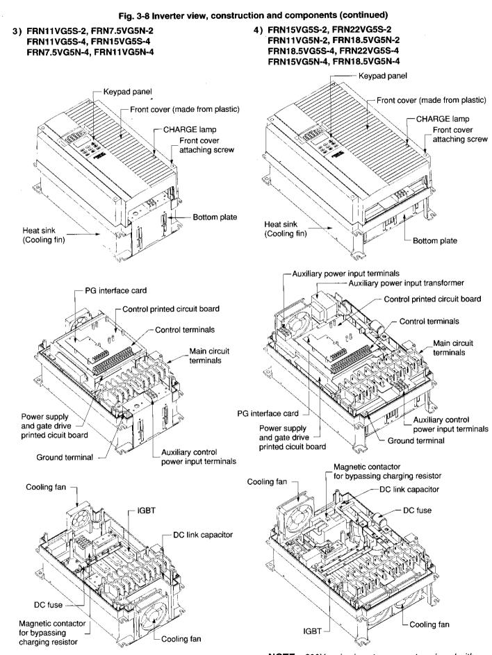
**NOTE :** 200V series inverters are not equipped with auxiliary power input terminals and transformer
