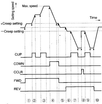
(1) By making FWD ON, the setting speed is accelerated in forward rotation up to + creep setting.
