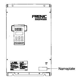
Fig. 2-2 Nameplate position
