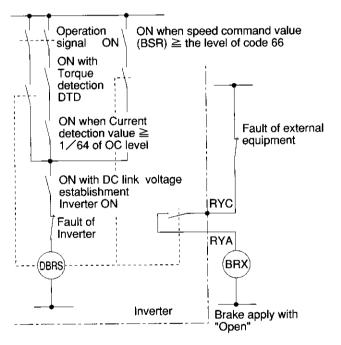
Write the torque level of releasing brake in the function "73 Torque detection (Level)".
