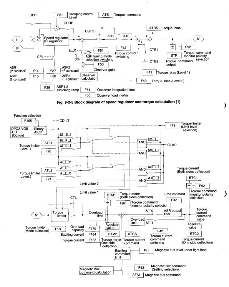
Fig. 9-2-6 Block diagram of torque calculation (2)
