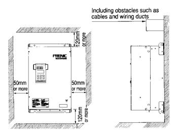
Fig. 5-2-1 Inverter mounting direction and clearance
