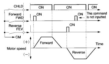
The coast-to-stop signal is valid even during operation signal holding.
