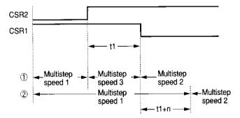
When the switchover timing between CSR1 and CSR2 is delayed for t1 (ms) as the operation example, without the agreement timer, the speed setting is switched from multistep speed 1 to multistep speed 3 and to multistep speed 2, then, a section of multistep speed 3 occurs (①). When the agreement timer is provided, this state is corresponded by setting the agreement timer for t1+n (ms),  $n \ge 1$  (②).
