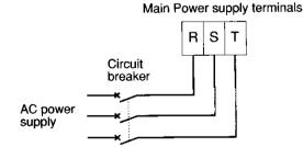
Fig. 6-2-1 Power supply connections
