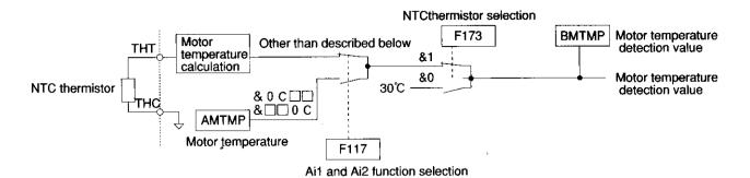
Fig. 9-2-7 Block diagram of motor temperature detection
