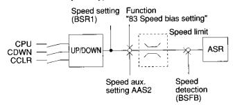
The signals of in acceleration or in deceleration are outputted according to increasing or decreasing of the UP/DOWN adjuster output BSR1.
