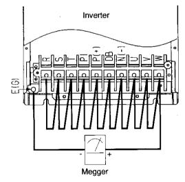
Fig. 11-4-1 Main circuit megger test connections
