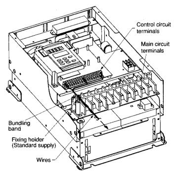
Fig. 6-5-13 Control circuit wire routing
