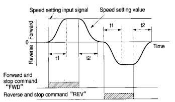
Acc/dcc. operation time from 0 to maximum speed (In the case of acc. time 1, dec. time 1 and S-curve acc/dec 1)<sup>•</sup>
