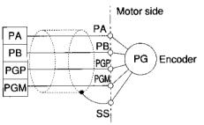
Fig. 6-5-10 Connection of encoder
