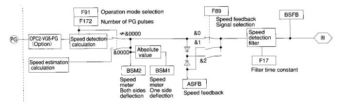
Fig. 9-2-4 Block diagram of speed detection section
