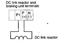
Fig. 6-2-7 DC link reactor connections
