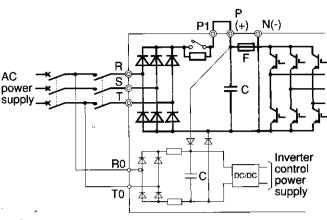
Fig. 6-4-4 Control power supply circuit
