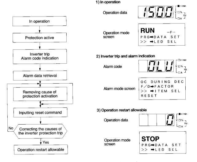
Fig. 12-1-1 Operation and indication at alarm mode
