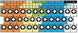
Orange = Outputs, Yellow = Analog Inputs, Blue = Digital Inputs
