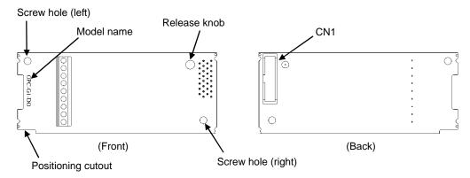
Figure 1.2 Name of Parts on Digital Output Interface Card (OPC-G1-DO)
