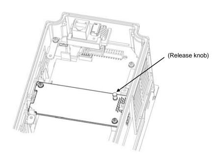
Figure 1.5 Mounting Completed (to B-port)
