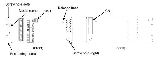
Figure 1.1 Name of Parts on Digital Input Interface Card (OPC-G1-DI)
