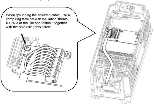
\* Pass the wires from the interface card between the control circuit terminal block and the front cover.
