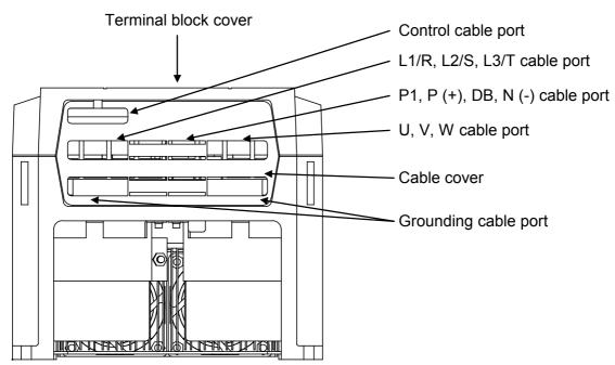
A barrier is provided in the cable cover for the P1, P (+), DB and N (-) cable port. Cut the barrier using nippers or the like before wiring.
