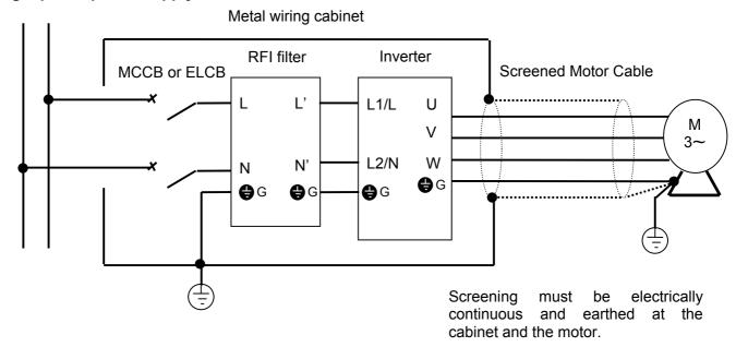
Fig.12-2-1 Recommended installation
