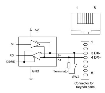
Fig. 9-4-1 Equivalent circuit of RS485 interface
