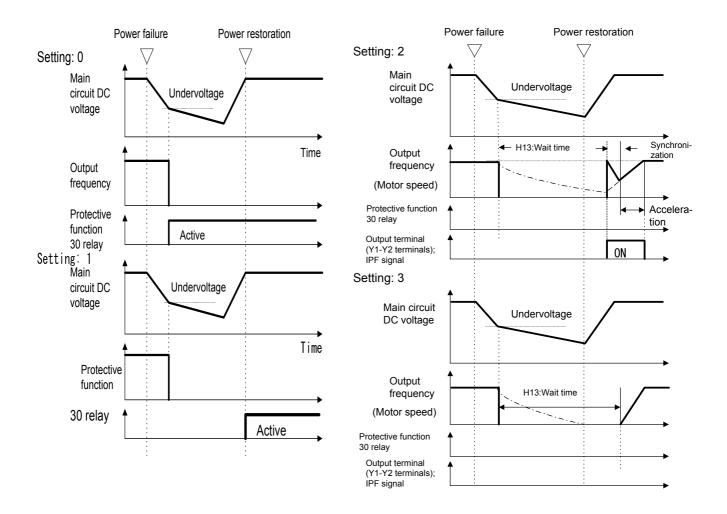
Note: The chain line indicates the motor speed.
