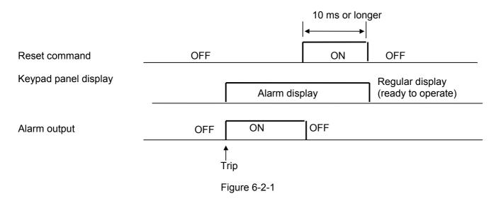
If an alarm reset is made with the operation signal turned on, a sudden start will occur. Check that the operation signal is turned off in advance.
