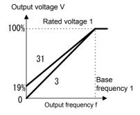
Note) When the torque boost value is excessively large, the motor is excessively excited in the low speed zone at all types of characteristics. If operation continues in such a state, the motor may be overheated. Set a value according to the characteristics of the driven motor.
