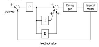
◆ Because forward and reverse operation can be selected for the output of the PID controller, the rpm of the motor can be increased or decreased in relation to the output of the PID controller.
