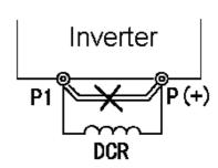
Fig. 2-3-1 DCR connection diagram
