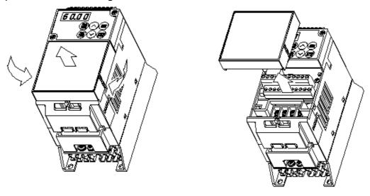
Fig. 1-3-1 Removing the control terminal block cover
