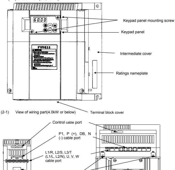
A barrier is provided in the main circuit terminal block cover for the P1, P(+), DB and N(-) cable port. Cut the barrier using nippers or the like before wiring.
