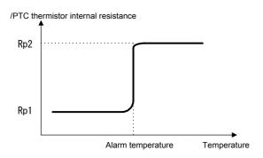
From the figure of H26 "PTC thermistor (Operation selection)", the 250-ohm resistor and the PTC thermistor (resistance Rp) configure a parallel circuit. Therefore voltage VC1 (operation level) of terminal [C1] is calculated in the following equation.
