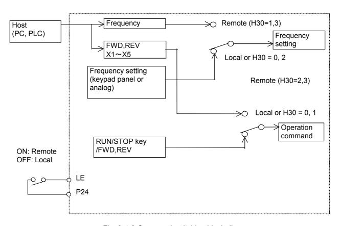
Fig. 9-4-3 Command switching block diagram
