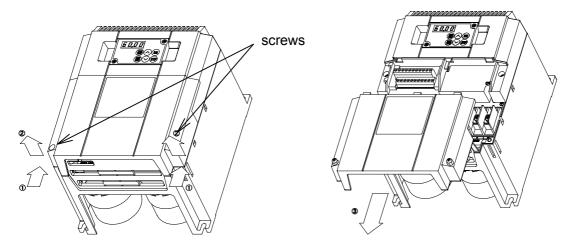
Fig. 1-3-3 Removing the terminal block cover
