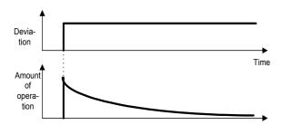
Setting range: 0.00 Inactive, 0.01 to 10.0 s D: differential time is used as a parameter to determine the effect of the D action. With a long differential time, decrease in the vibration caused by the P action upon deviation is quick. With too large a differential time, vibration may become larger. With a small differential time, decrease in the deviation becomes smaller.
