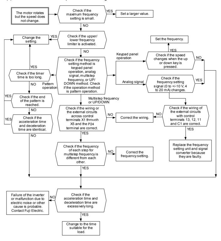
The change in the rotation speed of the motor is also small in the following cases.
