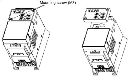
Fig. 1-3-4 Removing the keypad panel
