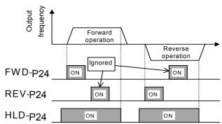
Note: The inverter operates while FWD-P24 or REV-P24 is ON even if HLD-P24 is OFF. An external interlock sequence ,which makes FWD-P24 and REV-P24 OFF when HLD-P24 is OFF, is required.
