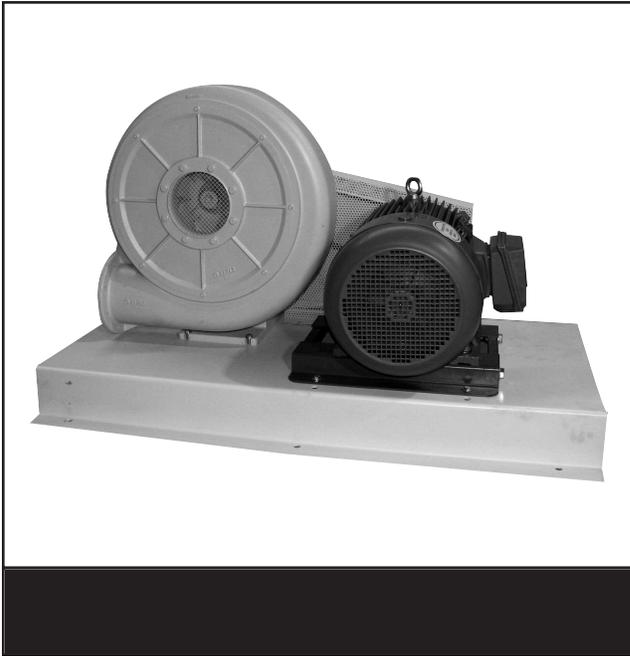
These Belt Driven Blower packages are provided with cast aluminum blower housings and aluminum closed impellers. The Blowers are provided in a clockwise rotation. Blower housing position may be changed from Horizontal to vertical discharge. Counter clockwise rotation may be provided. High performance V-belt pulley design provides compact design. All units are provided with mounting base and belt guard.
