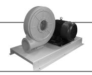
These Belt Driven Blower packages are provided with cast aluminum blower housings and aluminum closed impellers. The Blowers are provided in a clockwise rotation. Blower housing position may be changed from Horizontal to vertical discharge. Counter clockwise rotation may be provided. High performance V-belt pulley design provides compact design. All units are provided with mounting base and belt guard.
