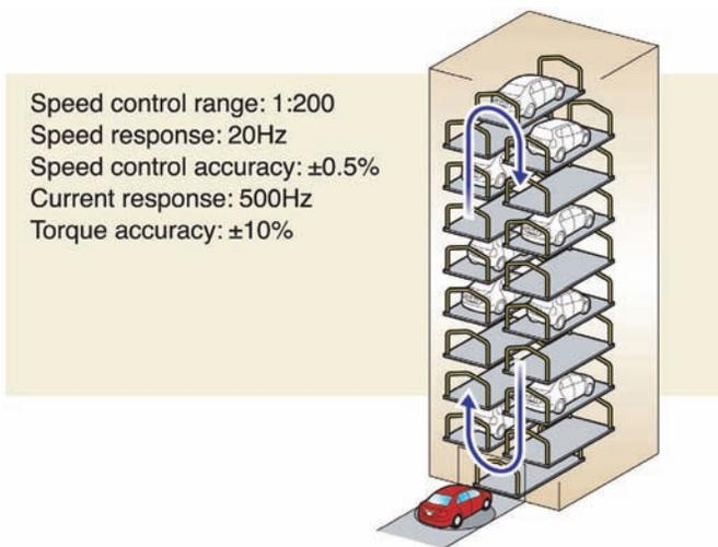
**Figure 3. Sensorless Vector Control**
