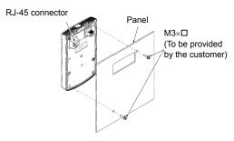
Figure 2.4 Mounting the Remote Keypad
