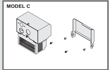
NEMA1 kit, when fitted to the FRENIC-Mini series, protects the inverter body with the structure that conforms to the NEMA1 standard (approved as UL TYPE1).
