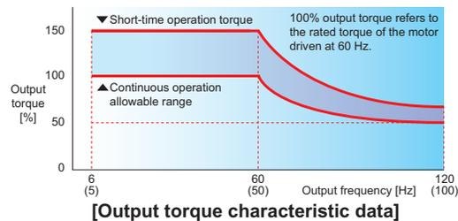
\*The above graph shows an example of torque characteristics obtained when FRENIC-Mini is combined one-to-one with Fuji's standard three-phase motor (8-type series; 4 poles).
