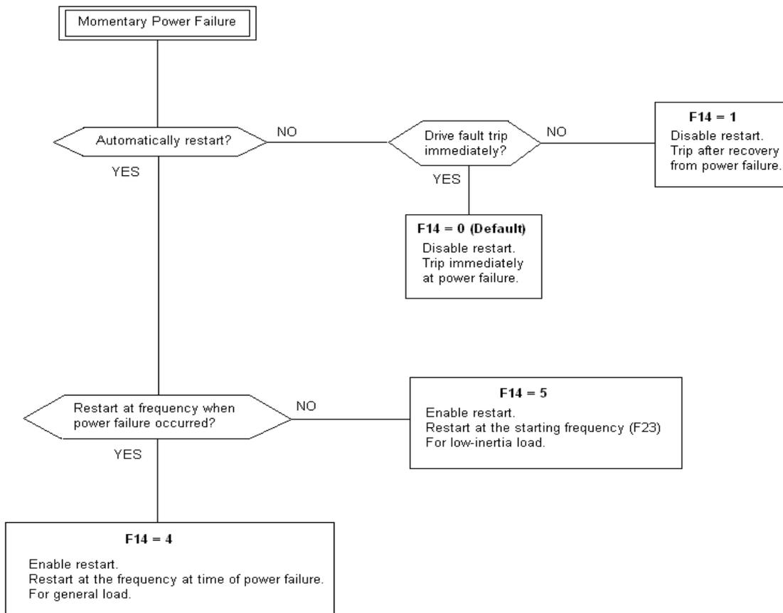
Note: “Momentary” power failure means power loss for only a few seconds, no longer than half a minute during operation.
