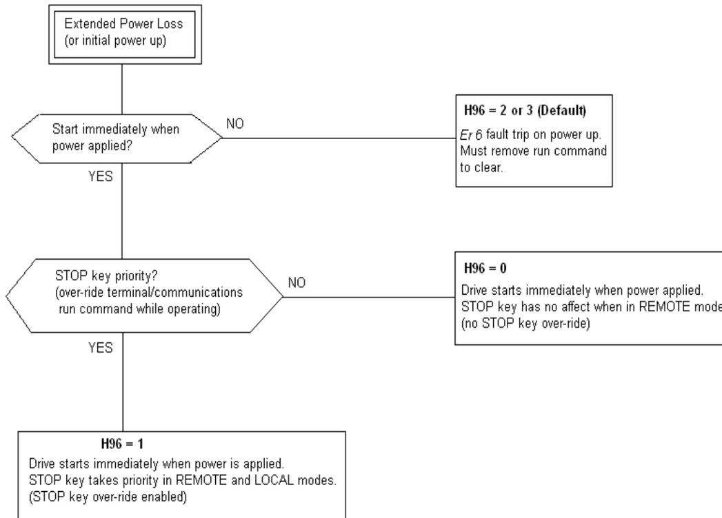
Note 1: In order for the drive to start operating immediately when power is applied (as displayed above), it must have a RUN command given by shorting the [FWD] or [REV] terminal with the [CM] terminal, and have parameter setting **F02 = 1**.
