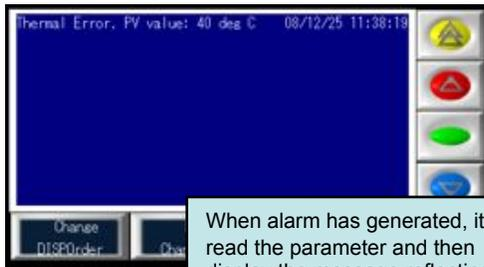
When alarm has generated, it will read the parameter and then display the message reflecting the registered content.
