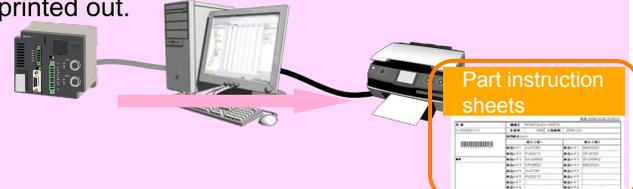
2)Based on the printed part instruction sheets, operators of each process pick parts and assemble them.
