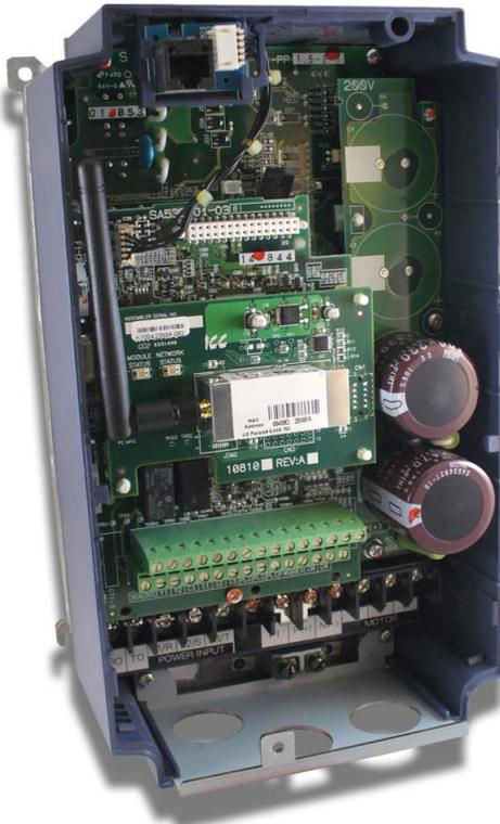
Figure 7: Example Installation Using Standard Dipole Antenna
