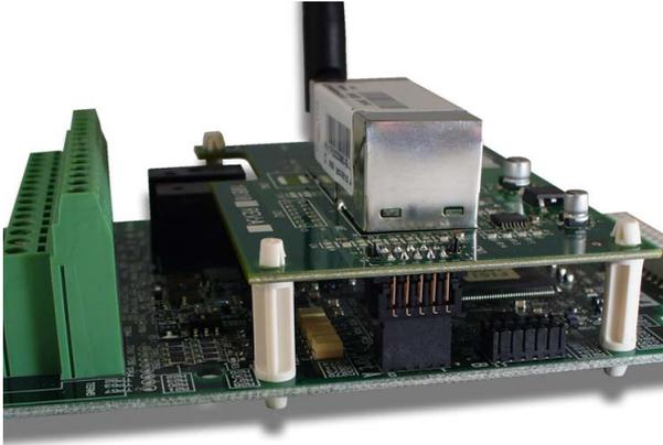
Figure 6: CN1 and "Port A" Connectors Properly Seated
