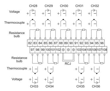
Note) For current input, connect optional shunt resitors to the voltage input terminals.
