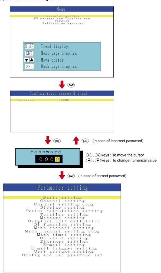
Note) After setting the parameters, select "Basic setting" / "Register data" in order to save the set information to a flash memory. To reset parameter set values, press OSP key. So, the following message appears. Press the ENT key twice. The parameter has been reset.
