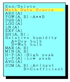
Move the cursor to the function you want to use and press the (ENT) key, and the following input data type selection screen appears.
