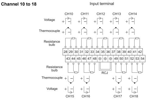
Note) For current input, connect optional shunt resitors to the voltage input terminals.
