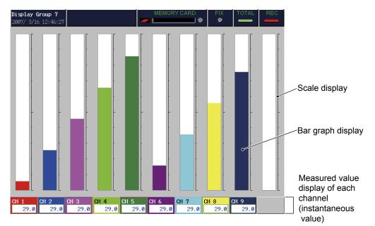
1. The measured data is displayed in a bar graph.
