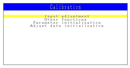
**CAUTION** Do not perform "Other functions" and "Adjust data initialization", since they are intended to be performed by the manufacturer. Otherwise the instrument may not operate properly causing phenomena that the input reading is not properly displayed or the set parameter returns to the value set at the time of delivery.
