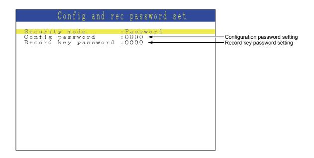
Press the (ENT) key, and password entry screen appears. Enter the password using the cursor key and press the (ENT) key.
