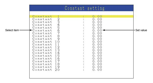
Enter the set value using the cursor key and press the  $(\ensuremath{\textit{ENT}})$  key.
