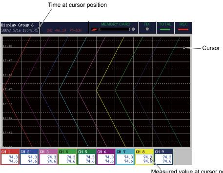
Measured value at cursor position of each channnel(Min and Max values)
