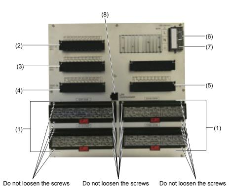
Note: Do not loosen the screws. Otherwise accurate measurement may not be carried out with thermo-couple input.
