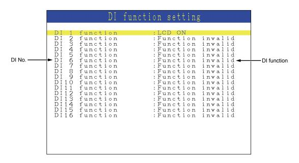
Move the cursor to the DI No. with which DI function is to be selected and press the *ENT* key.
