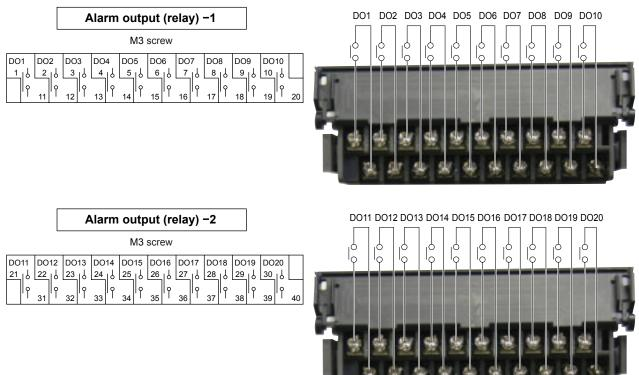
Note: If lamps are provided on the outside, set a resistor to prevent rush current. When relays or solenoids are used, set elements for contact protection (diodes or surge killers, etc).
