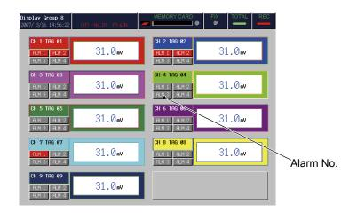
\* If an alarm occurs against the current input, the alarm contents are displayed on the historical screen and the record data display screen of the memory card. This is not the past alarm record.
