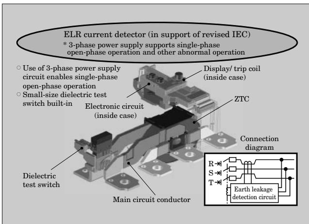
circuit tripped even in cases where one of the three phases is an open-phase. To support this requirement, a new small-size power supply circuit was developed and applied. In addition, ultra-miniaturization of the trip coil and modularization of mechanical parts that transfer motion enabled the successful development of a small-size earth leakage trip unit. (See Fig. 16.) As a result, the product was commercialized without having to modify the external dimensions of conventional products.
