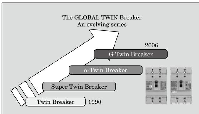
more product variety leads to more cumbersome selection and procurement of equipment, users are requesting its improvement. Under these circumstances, Fuji Electric has moved ahead with innovative technical development for low voltage circuit breakers, and has developed a 125 to 400 AF “G-Twin Series” as a global MCCB/ELCB series. (See Fig. 1.)
