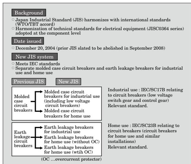
Fig.3 IEC harmonization in Japan, New JIS classifications
