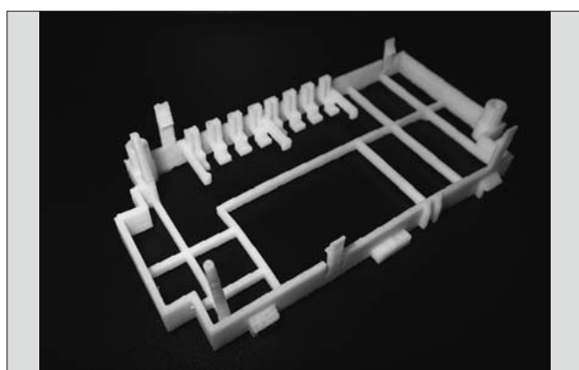
Fig.3 Example of 3D printer printout of power electronics equipment part
