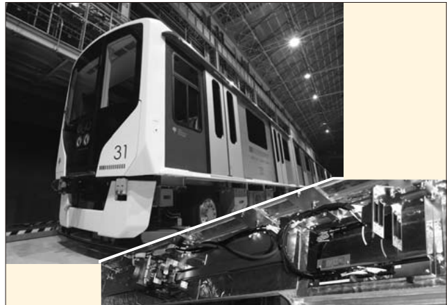
Fig.6 Model 330 cars and rack-and-pinion door drive system
