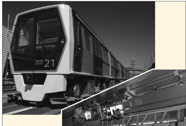
Fig.7 Series 2020 cars and rack-and-pinion door drive system
