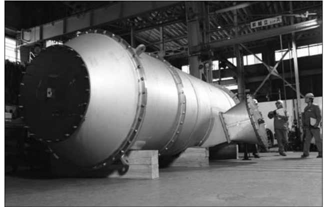
Fig.17 SO x scrubber for 9-MW main engine (diameter 2 m, height 6 m)
