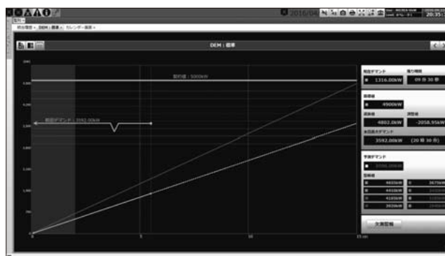
Fig.5 Example of demand monitoring screen
