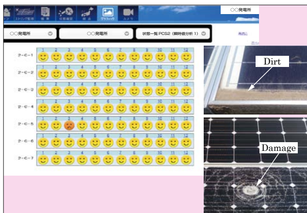
Fig.3 Example of screen of measurement system and abnormal condition of photovoltaic panels
