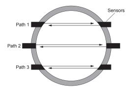
By measuring the flow with three parallel paths simultaneously, and averaging them, the flowmeter obtains the flow rate with  $\pm 0.2\%$  of rate accuracy.
