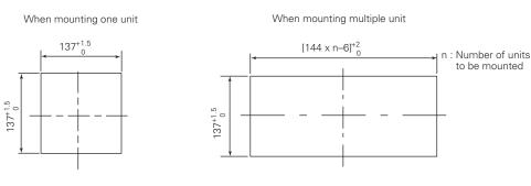
Note: When panel mounting, two bracket are necessary either on the top and bottom of the recorder.
