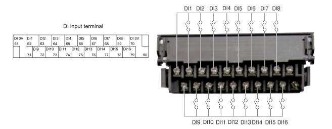
Note 1) DI (external control) unit is not insulated and should be used with a relay connected to the outside.
