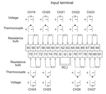
Note) For current input, connect optional shunt resitors to the voltage input terminals.
