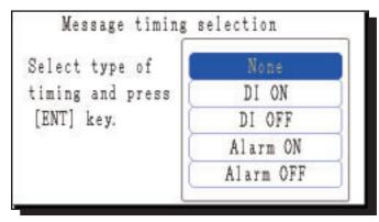
Select any item by the cursor key and press the  $\overline{(ENT)}$  key. After selection, the "Message Timing" screen appears as shown below. Set the "Channel" and "Alarm No." by the cursor key. After setting them, press the  $\overline{(ENT)}$  key for confirmation.
