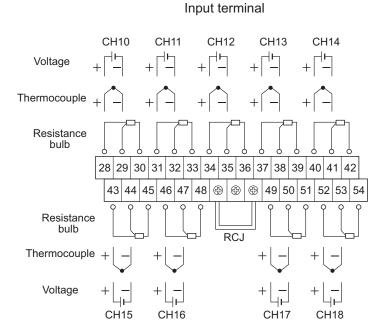
Note) For current input, connect optional shunt resitors to the voltage input terminals.
