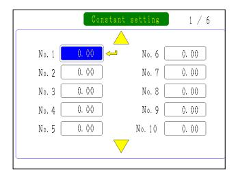
Move the cursor to the relevant constant No. and the constant setting screen appears as shown below. Enter the decimal point position and constant using the cursor key and (ENT) key.
