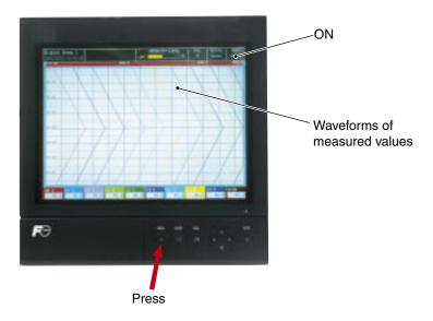
2) When the password for stopping and starting the record operation is set, the password setting screen is displayed as follows. Therefore, make a setting of the password. When the password is correct, the recording is started.
