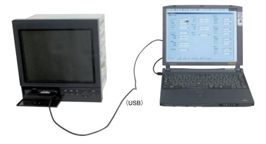
The loader cable should be connected to the USB port of PC.
