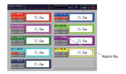
\* If an alarm occurs against the current input, the alarm contents are displayed on the historical screen and the record data display screen of the memory card. This is not the past alarm record.
