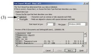
(4) Pressing the "Next" button displays the following screen.Check "Comma (C)" in the dividing character setting.
