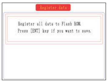
To save set values to the internal memory, press the  $\overbrace{\text{ENT}}$  key.
