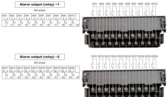
Note: If lamps are provided on the outside, set a resistor to prevent rush current. When relays or solenoids are used, set elements for contact protection (diodes or surge killers, etc). About alarm output (transistor)
