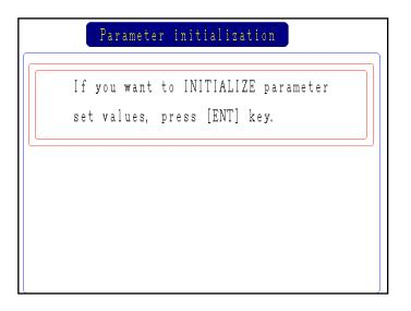
(3) Press the *ENT* key to return the parameters to the values set at the time of delivery from the factory.
