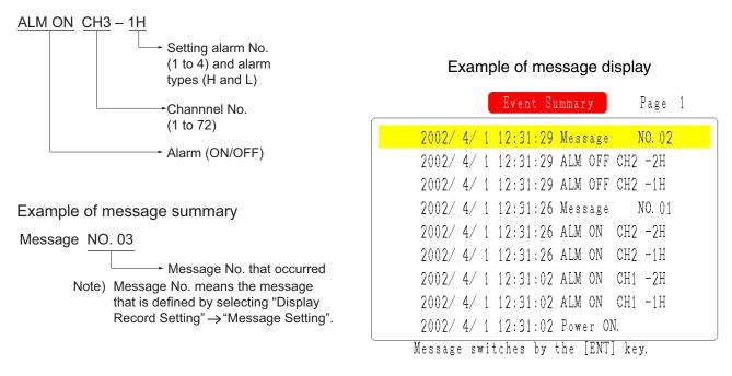
(7) Turn OFF/ON the power, and event summary is displayed. Message is changed according to recording status.1) When power is turned OFF/ON while recording is suspended
