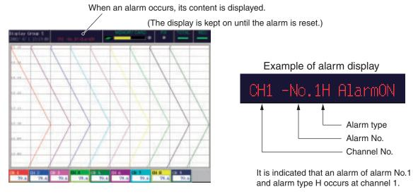
\* If an alarm occurs on the "Digital Display" screen, Alarm No. at left of "Measured value display" comes on in red.
