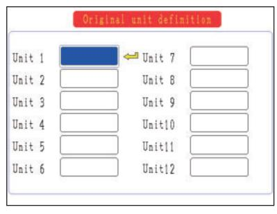
Move the cursor to the unit box that remains blank by the cursor key. By pressing the (ENT) key, the "Unit Naming" screen appears.
