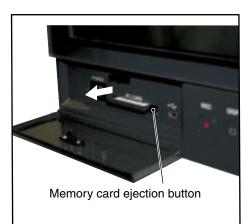
(3) Be careful with static electricity when removing the memory card.
