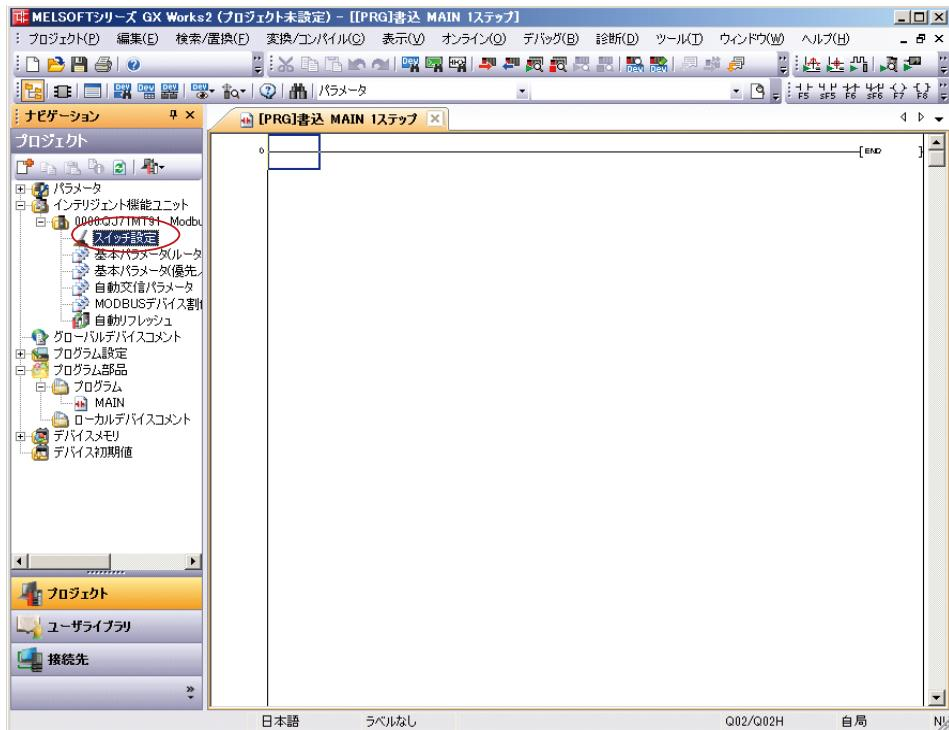
2. Enter the mode setting, transmission setting, communication speed for CH2, and station number setting for CH1/CH2, and then click OK.
