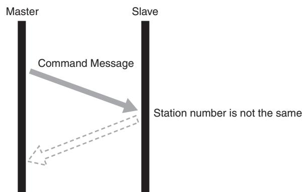
The master can communicate with an individual slave when multiple slaves are connected on the same circuit by the station number specified in the master's command message.
