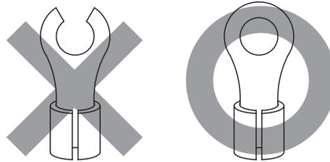
Attach the solderless terminals to the grounding terminals with them between the tooth lock washer and screw with washer.
