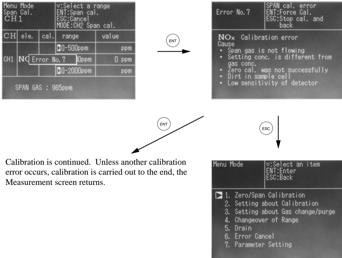
Calibration is continued. Unless another calibration error occurs, calibration is carried out to the end, the Measurement screen returns.
