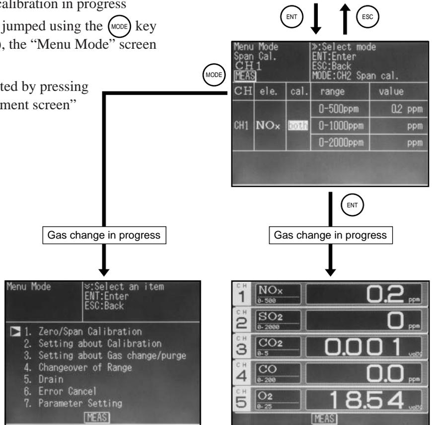
2) Exiting manual zero/span calibration in standby mode
