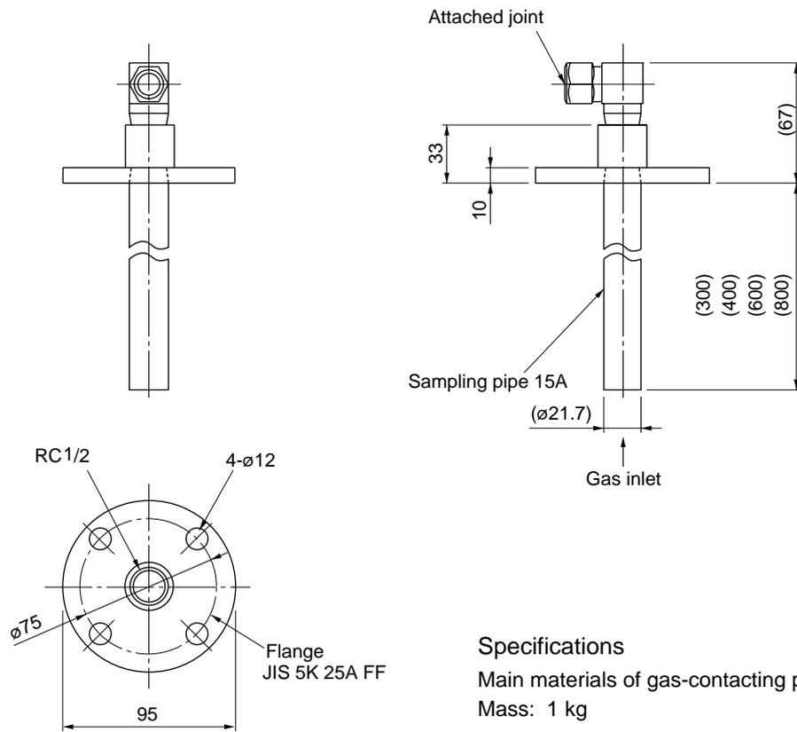
Attached joint (for  $\phi 6$  pipe connection)
