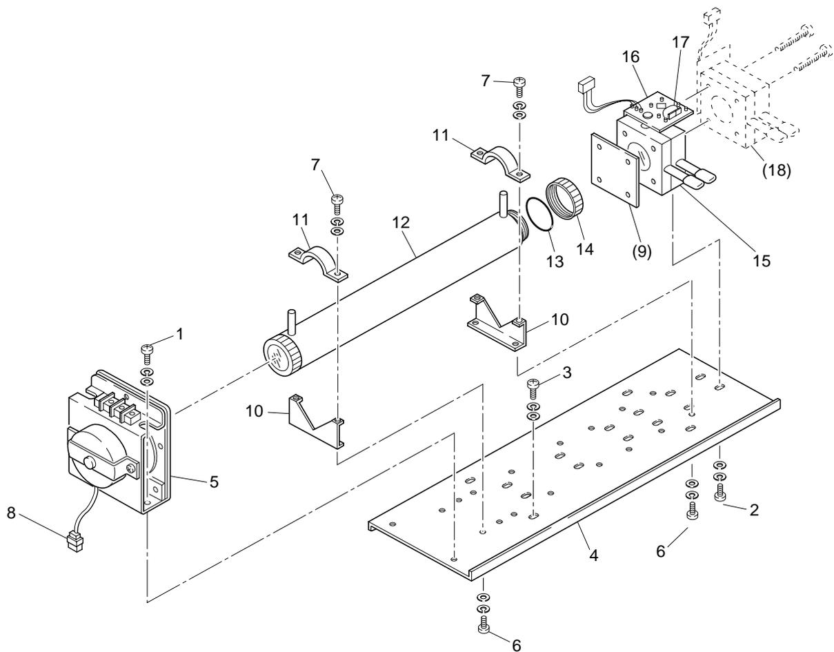
Fig. 5-1 Composition of measurement unit (pipe cell)
