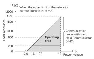
Note 1 : The load resistance varies with the upper limit of the saturation current [I max]
