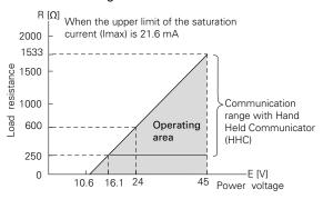
Note 1 : The load resistance varies with the upper limit of the saturation current [I max]
