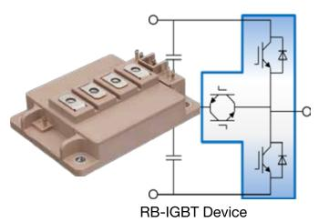
Fuji Electric UPSs use AT-NPC (Advanced-Type Neutral-Point Clamping) featuring our exclusive RB-IGBT (reverse-bias integrated bi-polar transistor):
